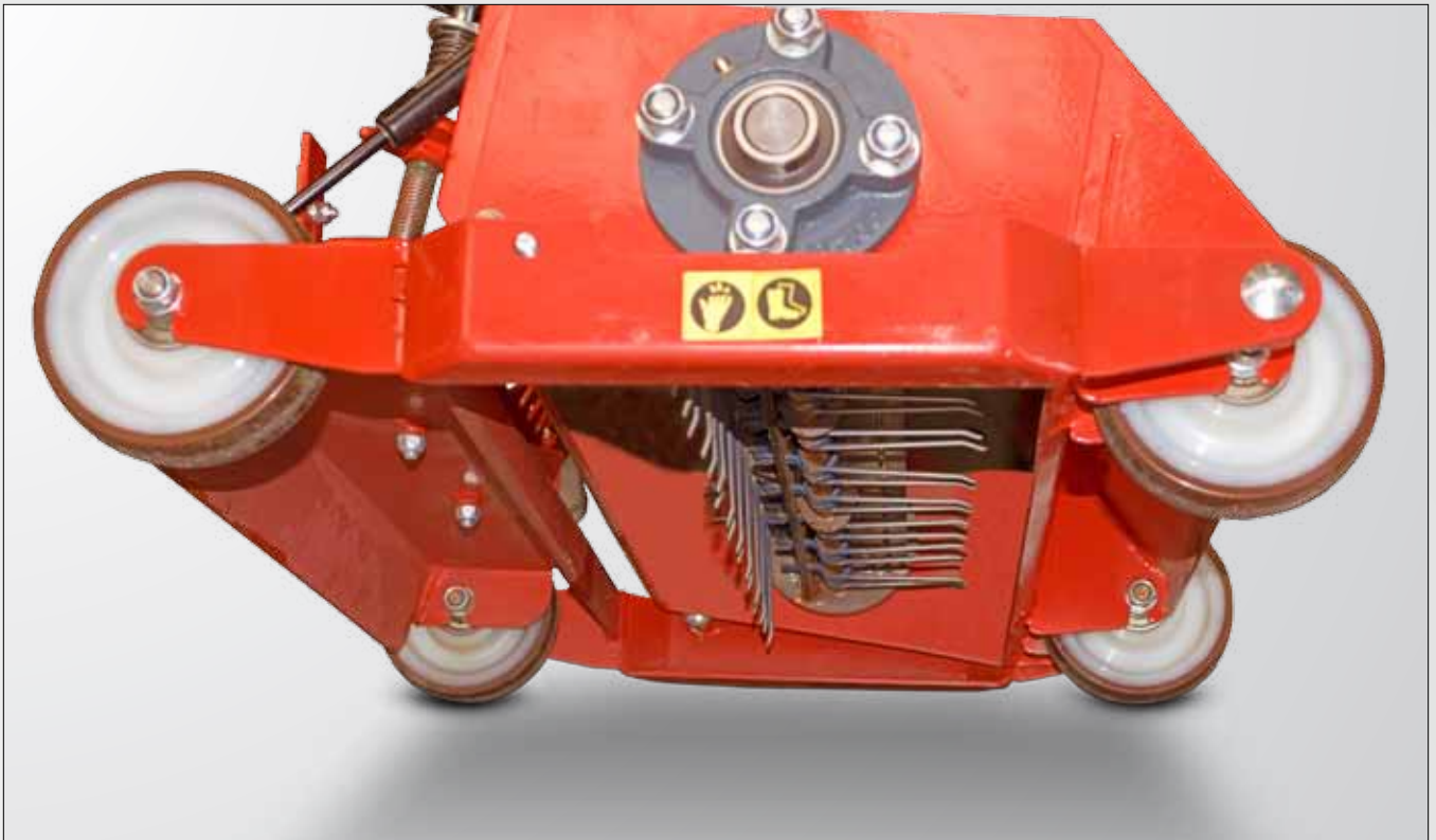
Rotating shaft with flexible prongs
